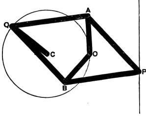
others at Q, and to the board at C, the end Q can be made to move on the circumference of a circle. If C be so placed that CQ is equal to CO, then, as Q is moved about, P will go accurately along a straight line.
